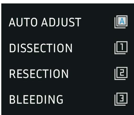
**Auto Adjust** is a system profile for setting the camera mode to automatically adjust the exposure and gain according to the lighting conditions.
