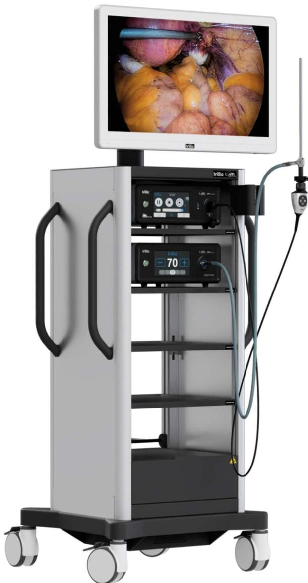
Irilic L.nm Laparoscopic Imaging System captures and displays real-time colour images in 4K resolution obtained in-vivo during surgical procedures.
