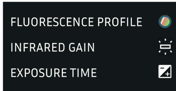
**Fluorescence Profile** opens allows users to change the Fluorescence Fusion Overlay colourmap.
