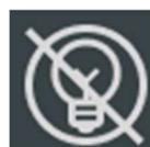
**Light Source Warning** – This symbol indicates that due to some issue the Light Source is not operational at expected levels. This may be due to wear and tear or some other form of damage to the LEDs. Please contact Irillic to schedule a visit by an authorized Service personnel to rectify this issue.
