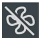
**Fan Error Warning** – This symbol appears when the cooling fan within the Light Unit is not operational. This may be due to some internal failure of the fan or even due to some obstruction preventing its operation. This can lead to catastrophic failure of the Light Unit due to overheating. Please contact Irillic to schedule a visit by an authorized Service personnel to rectify this issue.
