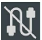
**Light Guide Connection Warning** – This symbol appears when the Light Guide is disconnected or dislodged from the Light Unit. This will also cause the light source to automatically power down to prevent any accidental emission of high intensity white light or infrared radiation. Please ensure the Light Guide is securely connected to the Light Unit by following the steps described in Chapter 6 of this manual.
