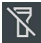
**Interconnect Error** – This symbol indicates that the WLU / FLU is not connected to the CCU via the Interconnect Cable. This Error State means that AMVI Mode cannot be enabled. The Interconnect Cable must be used to connect the WLU / FLU to the CCU as per the connections described in Chapter 6 of this manual.
