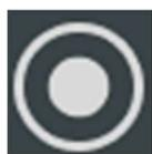
**Recording ON** – This symbol indicates that the current live feed is being recorded onto the attached storage device. The saved video files will be named with the time stamp of the start of the recording. Videos will be captured in FHD resolution, while Images will be saved in the full 4K resolution that they are displayed in.
