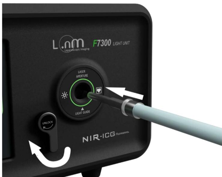
**Fig 6.3: Light Guide to Light Unit Connection**
